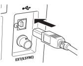
Communication interface in this instrument conforms to USB1.1. Hold the USB cable plug in unplugging. Do not pull the cord. Plug the USB cable to fit the connector entry point.
