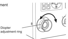
Adjust so that A or B on aperture or black circle indicating measuring area looks clear when observing object through finder. Adjustment would be easy starting with 1° aperture where object near aperture looks blur.
